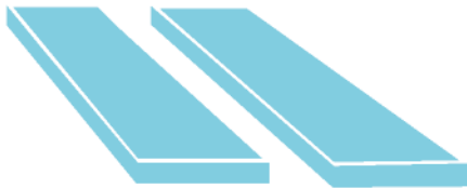
Hot Rolled Strip (by Gas Cutting or Sher Cutting)
